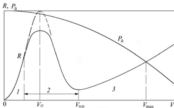
Fig.4. Dependence of drag and available thrust on velocity
